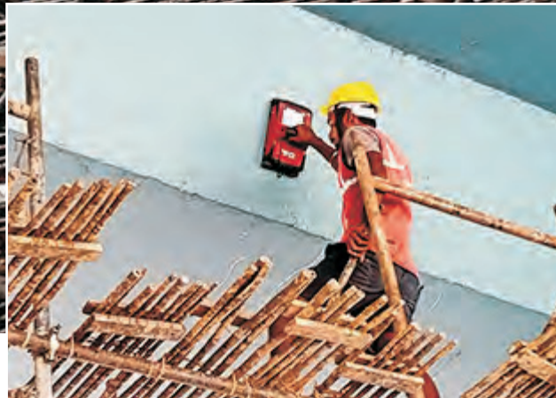
Reinforcement Scanning by Using GPR Machine
